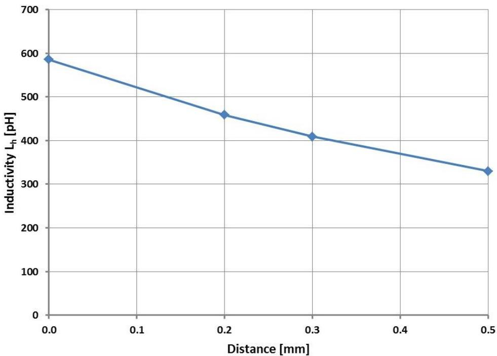
Figure 14: Main inductance  $L_h$  of the BS 06DU-s field source dependent on the distance  $h$  to the conductor at current  $i_P$  of 20 A.
