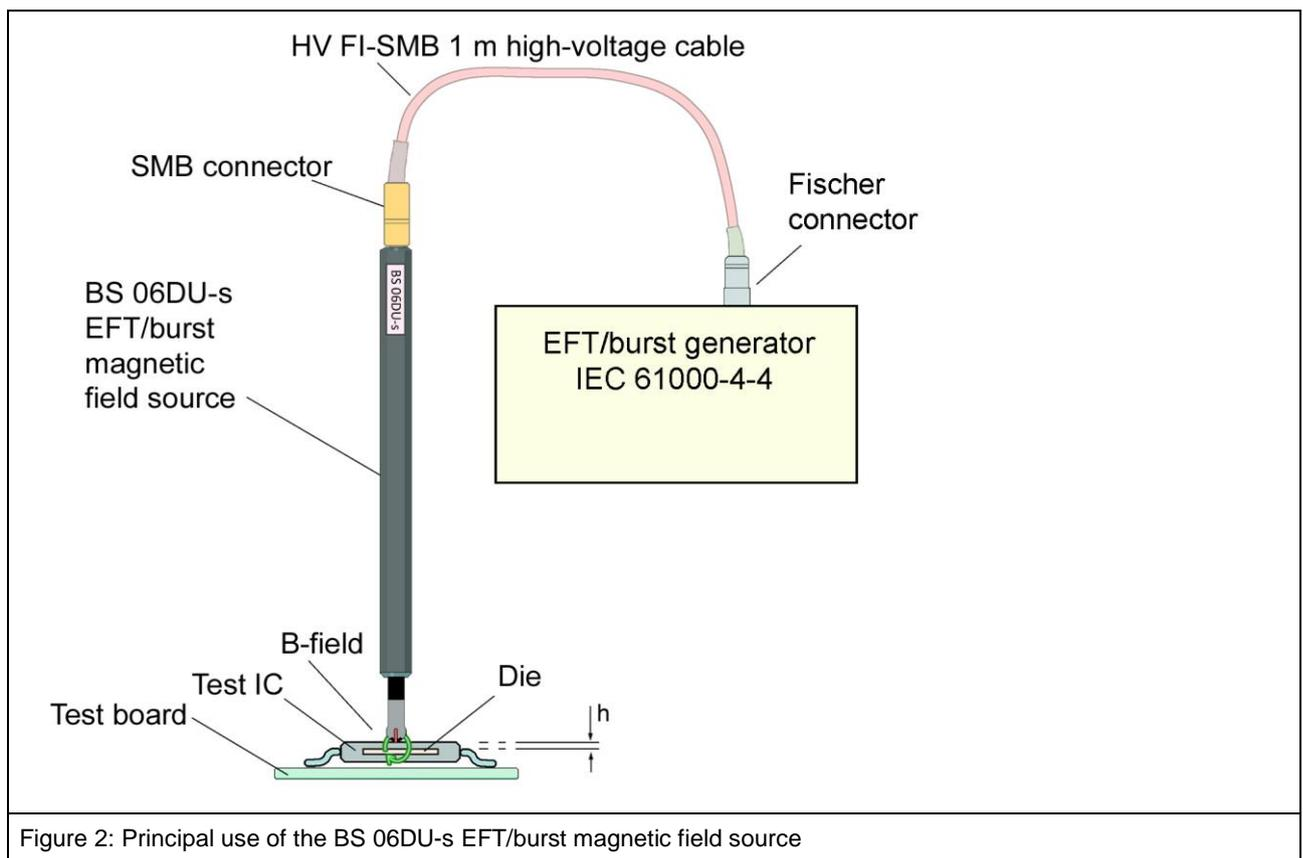
Figure 2: Principal use of the BS 06DU-s EFT/burst magnetic field source
