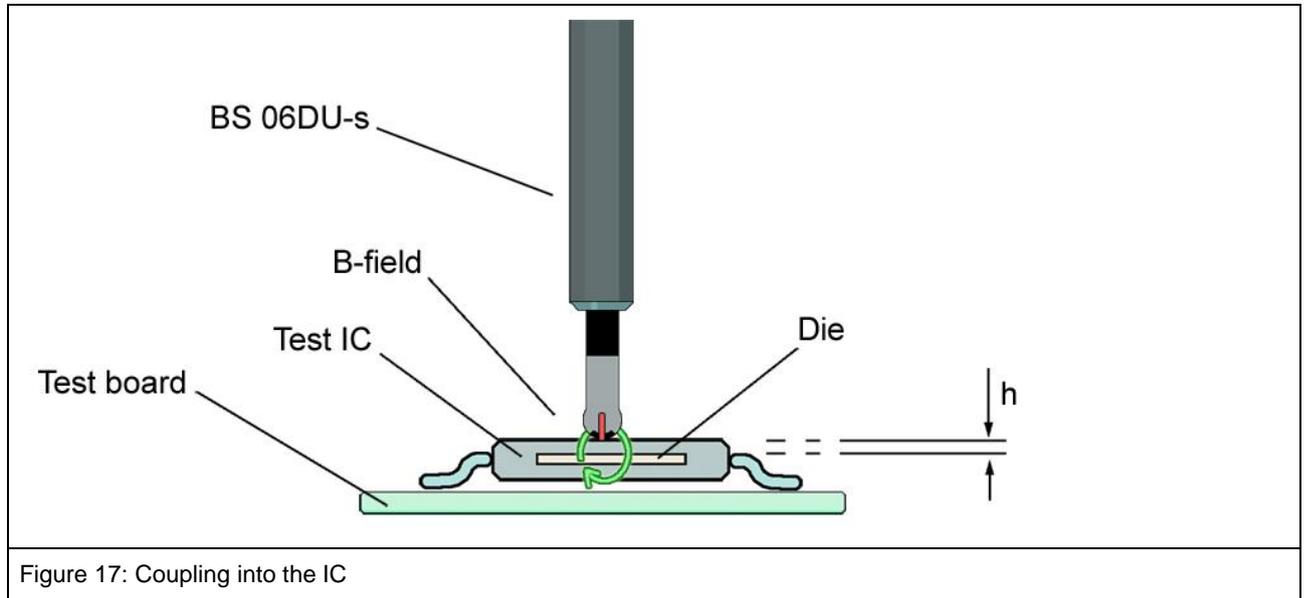
Figure 17: Coupling into the IC
