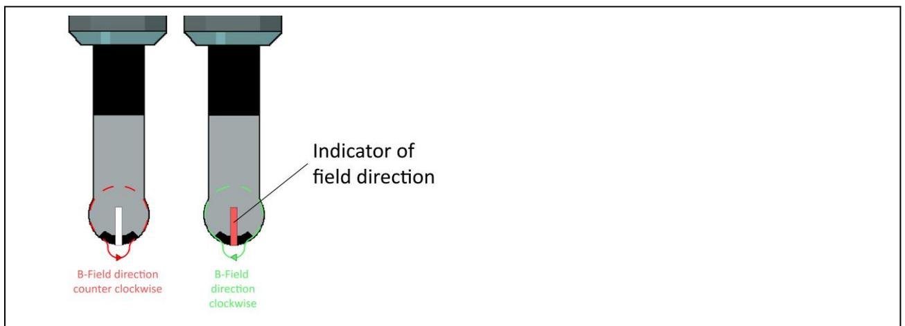
Figure 10: Assignment of the magnetic field direction with positive polarity of the EFT/burst generator
