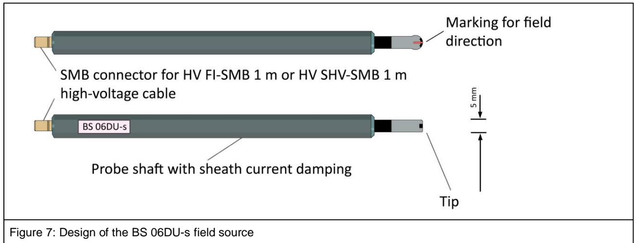
Figure 7: Design of the BS 06DU-s field source
