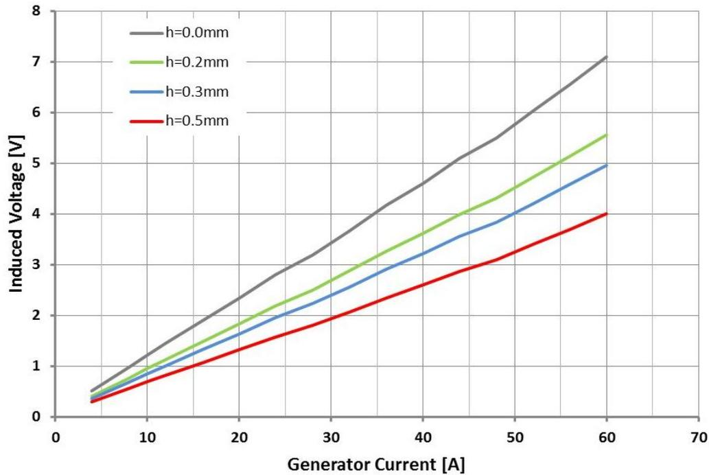
Figure 13: Induced voltage ( $U_{ind}$ ) of BS 06DU-s as a function of generator current. Parameter is the distance  $h$  of the field source from the measuring point.
