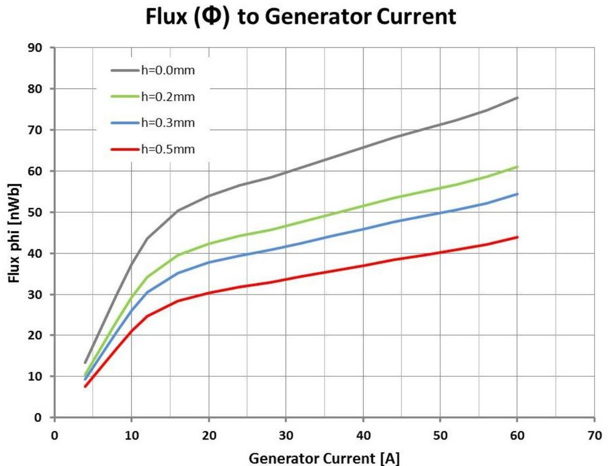
Figure 12: Flux  $\Phi$  provided by the BS 06DU-s field source as a function of the generator current. Parameter is the distance  $h$  of the field source from the conductor.
