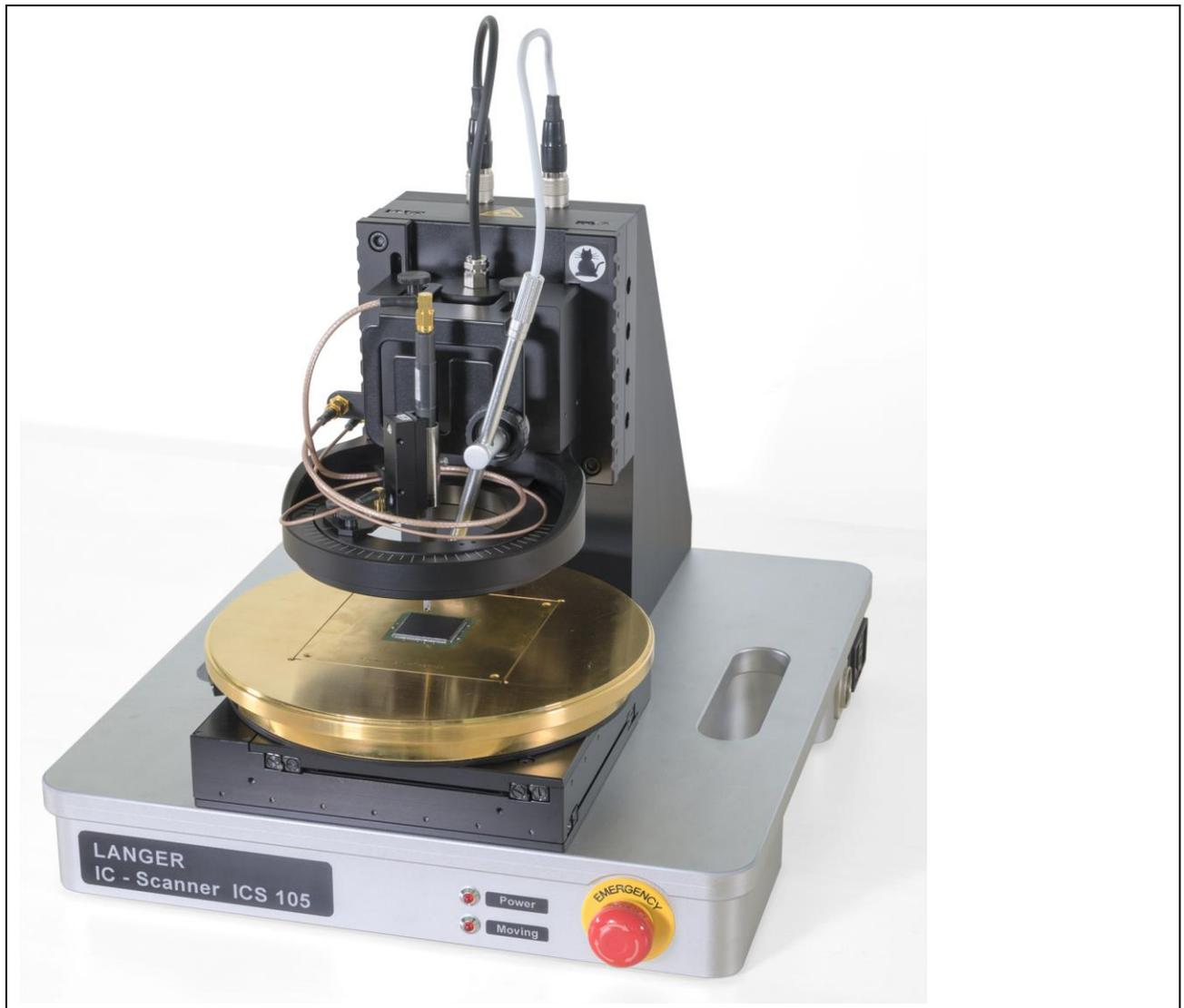
Figure 3: Use of the BS 06DU-s EFT/burst field source in conjunction with the ICS 105 IC scanner and ICE1 set components
