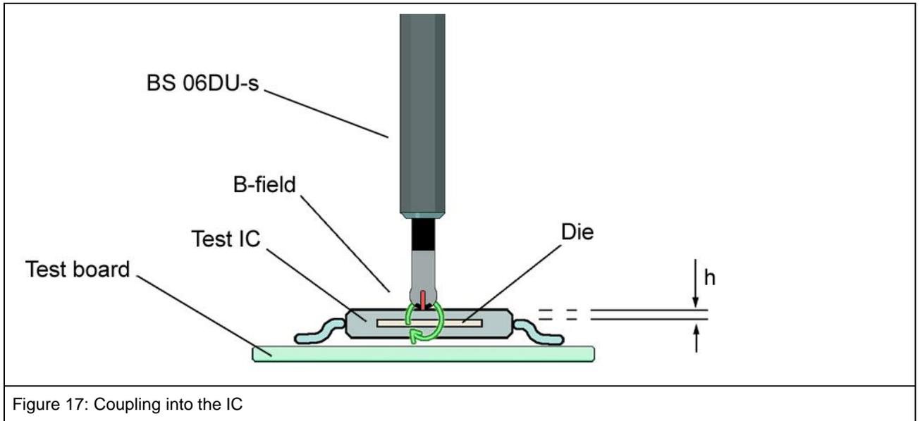
Figure 17: Coupling into the IC
