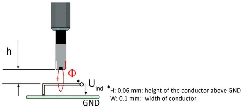
Figure 11: Assignment of the magnetic field direction with positive polarity of the EFT/burst generator
