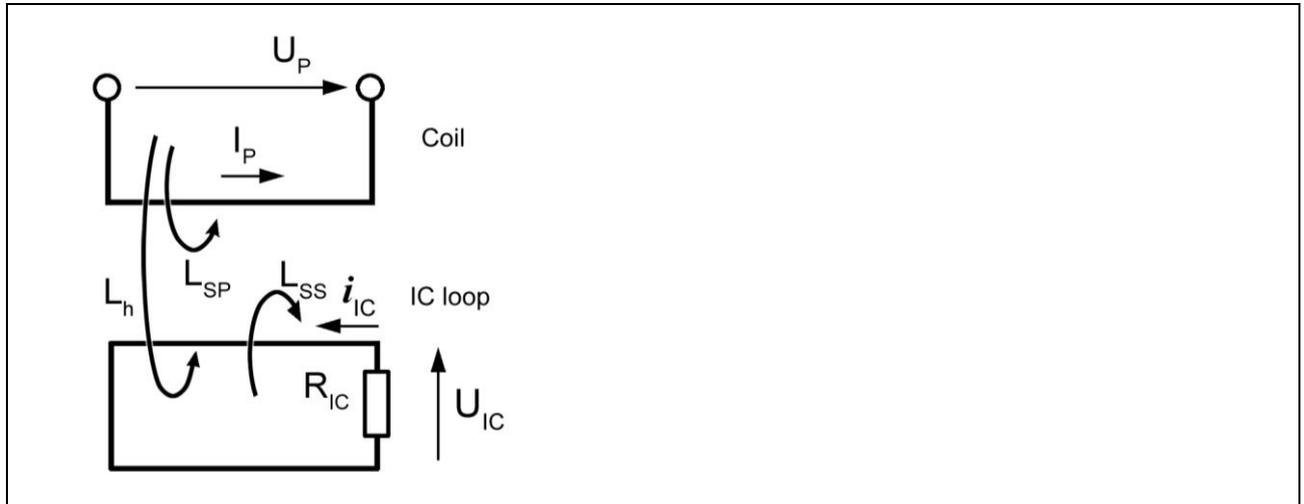
Figure 15: Flux equivalent circuit diagram of the BS 06DU-s field source's coil and the IC loop.
