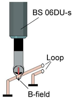
Figure 20: Coupling to a vertical loop / conductor
