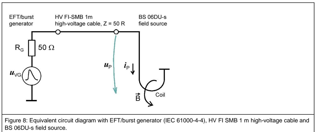
Figure 8: Equivalent circuit diagram with EFT/burst generator (IEC 61000-4-4), HV FI SMB 1 m high-voltage cable and BS 06DU-s field source.
